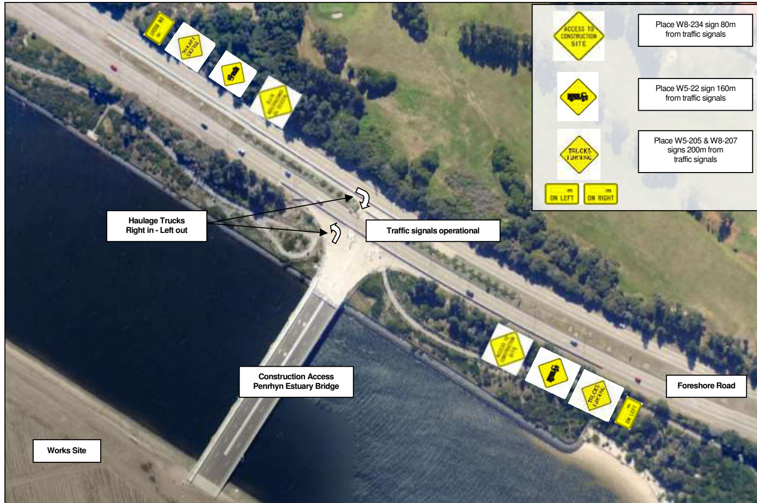
Figure 6 Access Intersection and Signs
