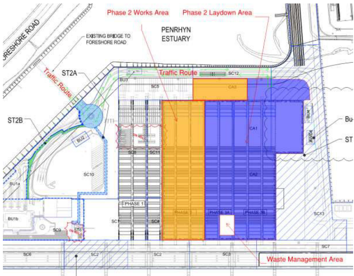
Figure 1 : SICTL Terminal 3 Phase 2 works and laydown area
